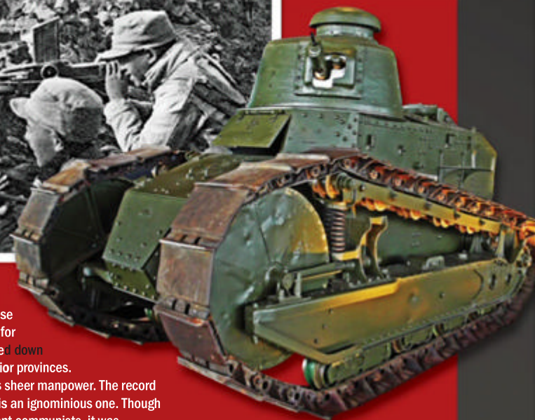
Above: The National Revolutionary Army had its own small armoured corps using the French Renault FT-17 light tank
